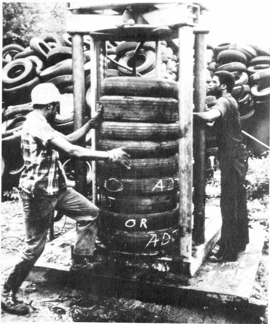
Figure 12.—The ten-tire bale is assembled by compressing ten tires into a bale, which is held together by steel and plastic bands.
